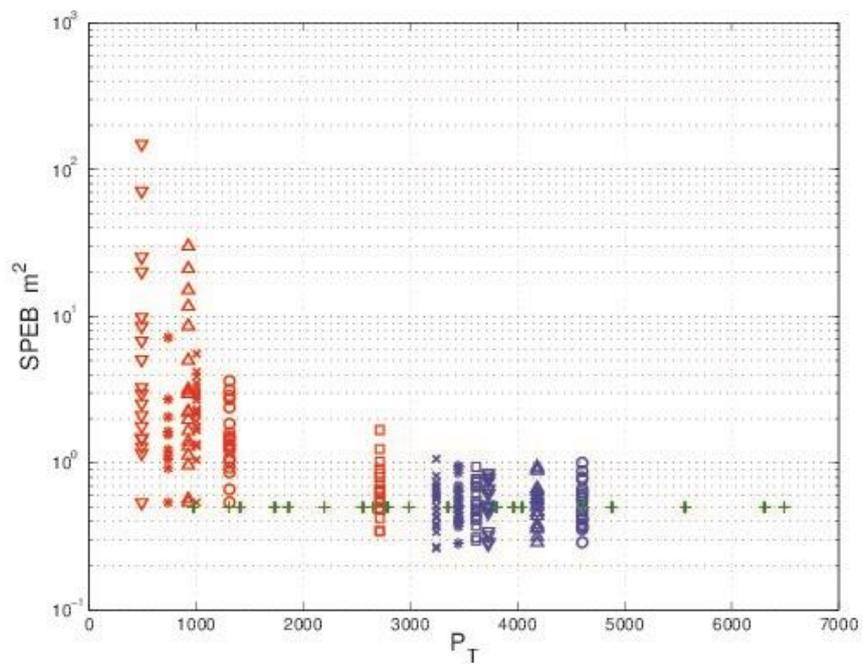
The above figures show the required total power for all the anchors to satisfy the SPEB constraint for multicast and unicast methods based on ergodic (blue) and non-ergodic designs (red) for several channel coefficients before the movement.
