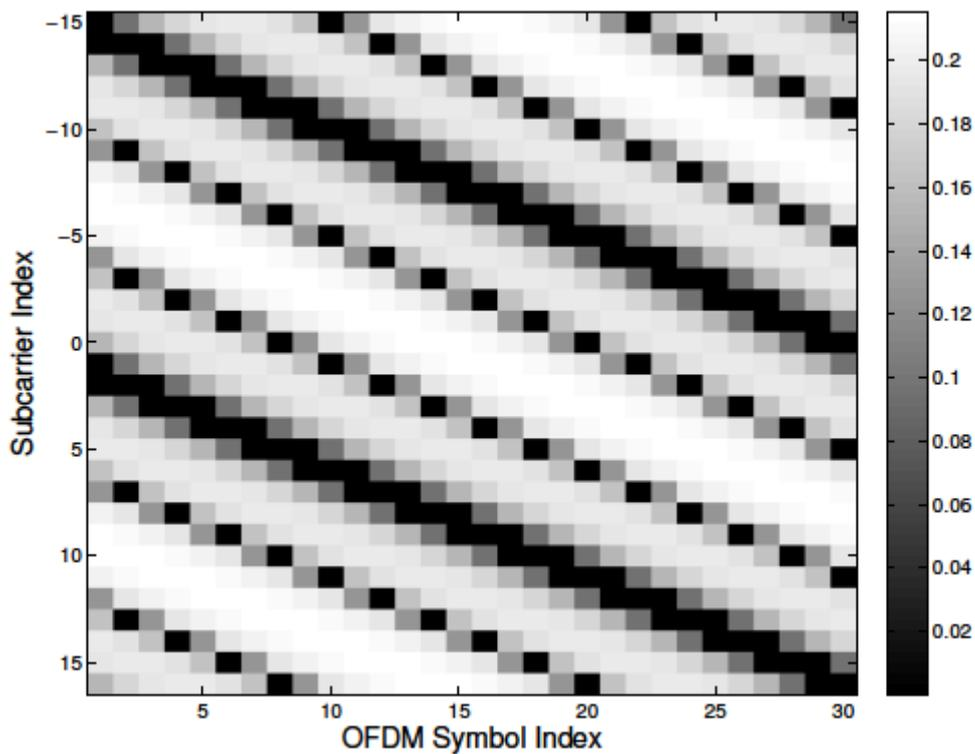
Fig. 1. Joint Data and pilot allocations in a block-fading time-varying OFDM system.
