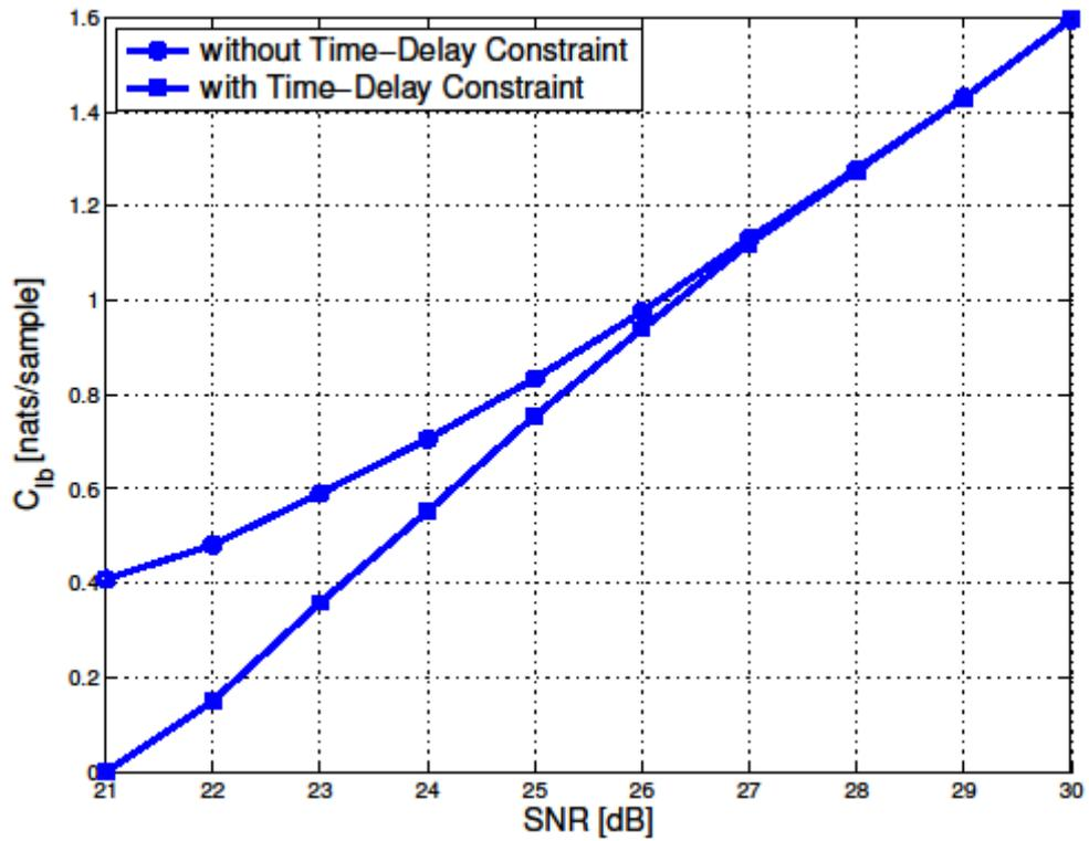
Fig. 4. Channel capacity versus the SNR with and without time-delay constraint.
