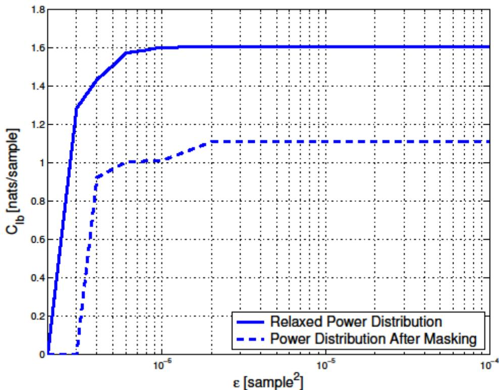
Fig. 2. Channel capacity versus the upper bound of time-delay estimation accuracy.
