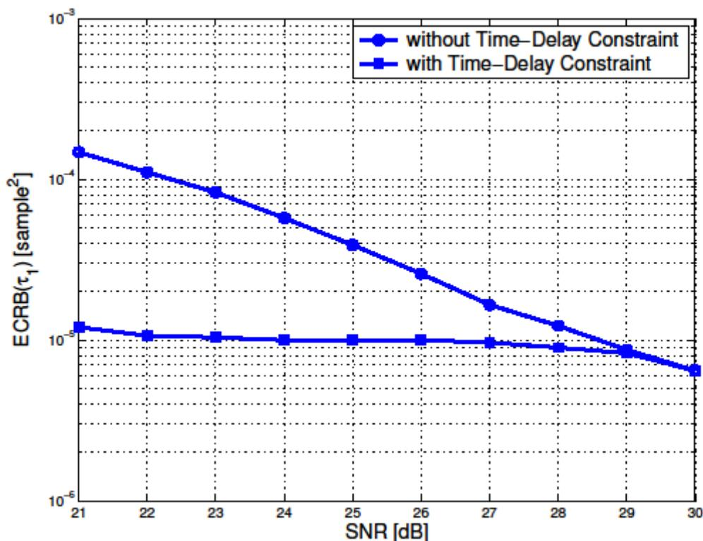
Fig. 3. ECRB of time-delay versus SNR with and without applying time-delay constraint in the optimization.
